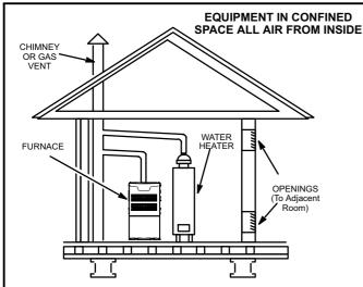
NOTE - Each opening shall have a free area of at least one square inch (645 mm<sup>2</sup>) per 1,000 Btu (.29 kW) per hour of the total input rating of all equipment in the enclosure, but not less than 100 square inches (64516 mm<sup>2</sup>).
